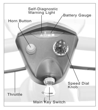
Figure 2 - EW-M39 Top Control Panel
